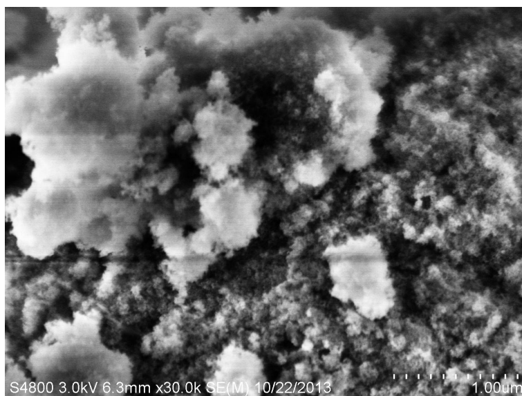
Typical SEM Image of ACS Material Diamond Nanoparticles
