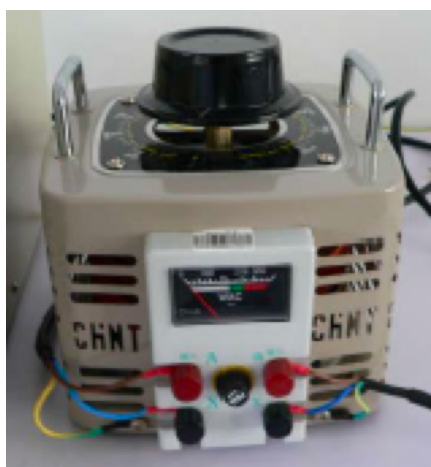
Photo of Voltage Regulator
