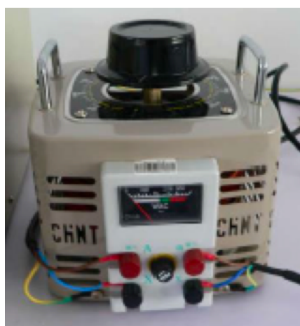
Photo of Voltage Regulator
