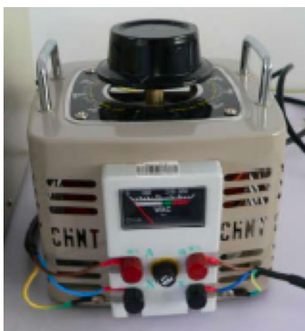
Photo of Voltage Regulator
